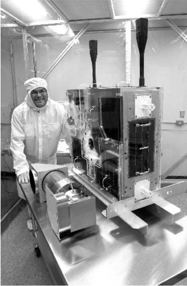
**Figure 3.10** The *Microvariability and Oscillations of STars* (MOST) satellite, and the Project Scientist Jaymie Matthews, in the ‘clean room’ of the Institute for Aerospace Studies, University of Toronto. The satellite is about the size of a large suitcase and, as the Project Scientist has pointed out, it weighs less than he does. (From MOST Science Team.)
